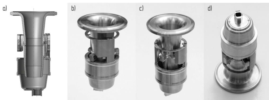
Fig.S3. Drawing (a) and photographs of the shutter: b) and c) movable mask locked in position for sample transfer and for deposition, respectively; d) upside down view showing the aperture of the mask.
