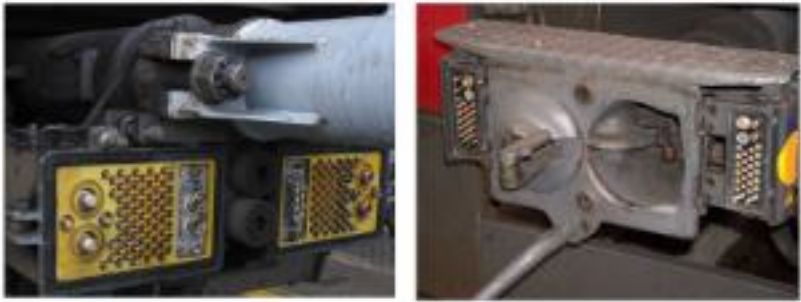
Figure 3.7: Photos of two different train coupler types showing electrical wired communication interfaces to transfer safety critical control data between wagons.
