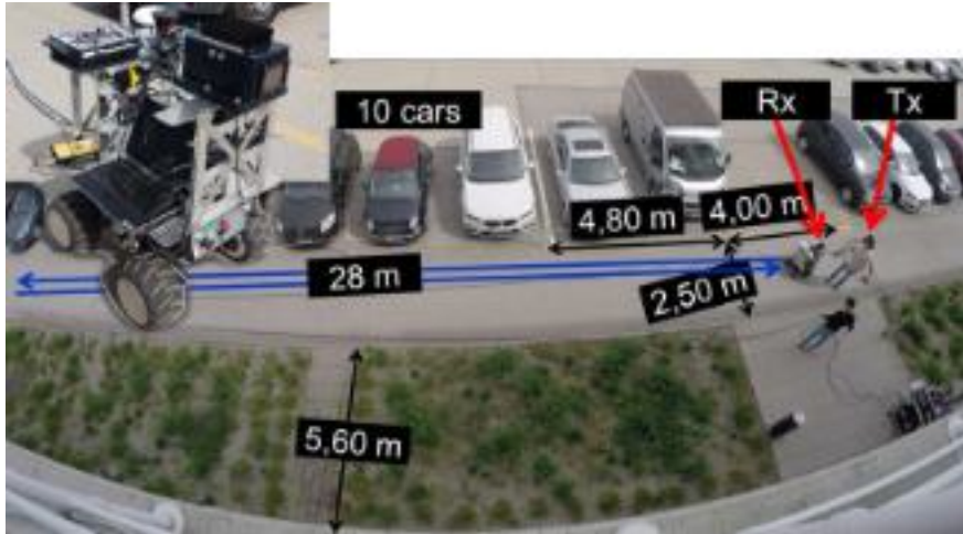
Figure 4.8: A top view shot of the dynamic tests environment. The receiver front-end was mounted on top of a remote-controlled rover (top-left corner) to enable dynamic measurements.
