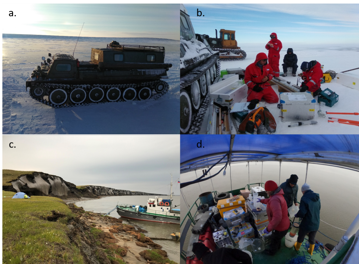
Figure 4-2. Sampling vehicles in winter and summer. a) all terrain caterpillar vehicle in the Lena Delta on the Lena Delta river ice for reaching field sites further from the camp; b) Working process on ice in the Lena Delta in winter: drilling and water sampling; c) The research vessel "Merzlotoved" with the Sobo-Sise Yedoma cliff in the background; d) Water sampling at the back of the research vessel in the Lena Delta in summer 2019.
