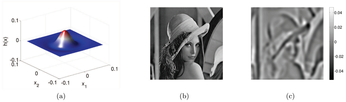
Figure 1.1: The filter kernel of the Mexican hat function ( \sigma = 0.025 ) is illustrated in (a). The filter response (c) of the image (b) is computed by the convolution of the image and the filter kernel.
