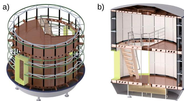
Fig. 1. (a) CAD-model of the basic MaMBA module, showing the interior structure of the pressure vessel (not the hull itself). It consists of 2 stories; the lower story has 3 doors, of which one is shown on the left. (b) Different view of the same model, showing the inner and outer vessel walls. The exterior wall is cylindrical, the interior wall consists of 18 segments. Both walls are min. 30 cm apart. In this view, one door is shown half on the left, another one is behind the stairs.
