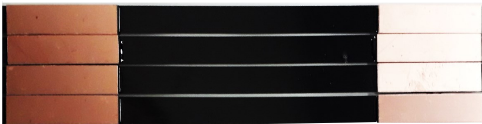
Fig. 8.4 Fiber composites for tensile test. a) Sample dimensions. b) Finished samples.
