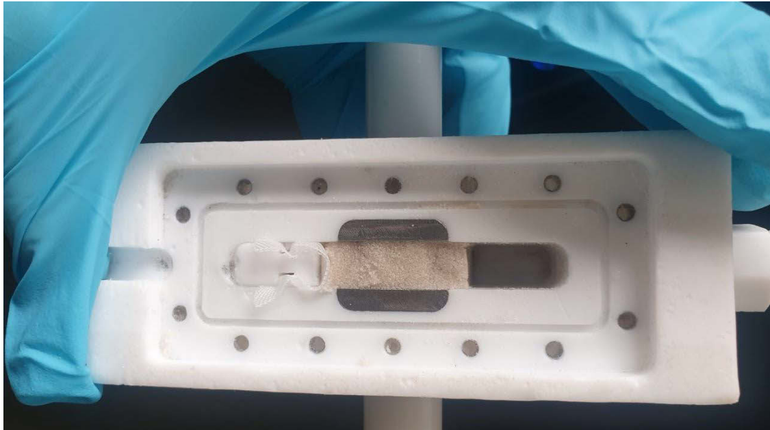
FIGURE A.2.1 Packed bed of sand inside the filter cell (located between two metal electrodes) 1 .
