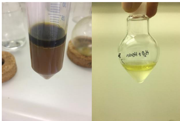
Figure. 107: Left: Separated green phase from the crude extract. Right: H 2 O and hexane liquid/liquid partitioning.
