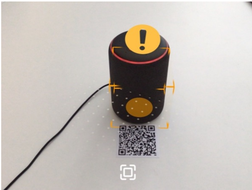
Figure 4.25: Upon scanning a QR code, the AR app displays a visual overlay over the actual physical device.
