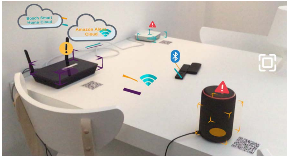
Figure 4.27: Upon scanning a device’s QR code and accepting the associated privacy policy, the chosen smart home device is integrated into the system. The corresponding cloud service is displayed prominently above the physical router in the AR scene. Animated dashed lines connect the device to the cloud, using dynamic color coding to enhance visibility and make the device-to-cloud relationships easier to understand and follow. Moreover, tapable icons indicating the communication protocol, such as Wi-Fi and Bluetooth, are displayed along these lines.
