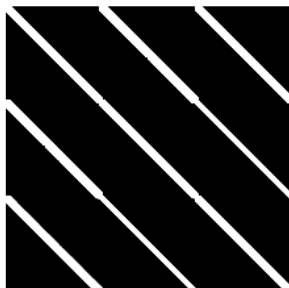
Figure 3.4: Visualization of the typical sparse banded structure of the stiffness matrix \mathbb{K}(\rho) . In the image, zero values are displayed in black, and non-zero values in white.
