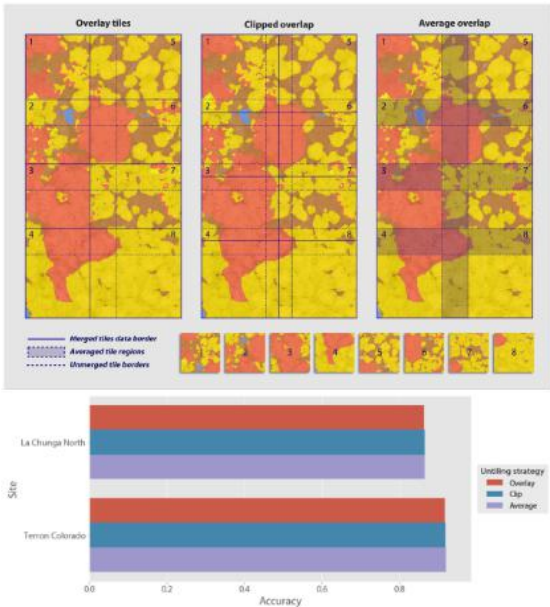
Figure 4.7 Semantic tile-merging strategies. For the semantic segmentation tiles we tried 3 different untiling strategies to recover the predicted habitat map: overlaying, clipping and averaging. We compared them to the ground truth densely annotated tiles and calculated their accuracies. No clear advantage was detected for any of the untiling strategies, which hints at the good prediction confidence of state-of-the-art semantic segmentation networks, even around borders of images.
