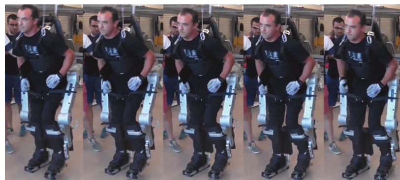
(e) ATALANTE lower limb exoskeleton with free hands during walking experiments with a paraplegic patient (photo credit: Wandercraft)
