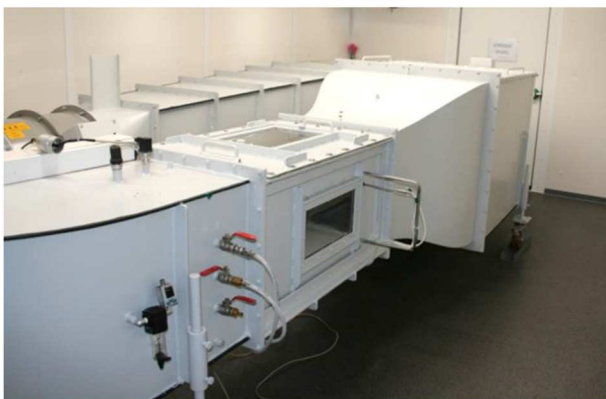
Figure 4: Photo of the climatic wind tunnel of DWG WTS. The 0.5 m × 0.5 m × 0.8 m test section with two windows, is located after the nozzle. Flow is from right to left.
