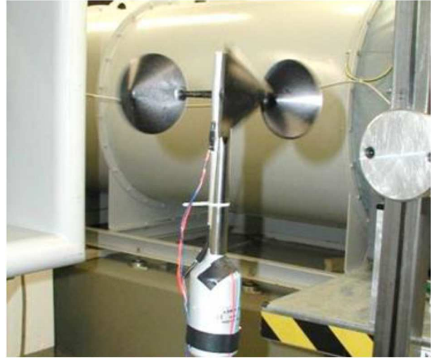
Figure 2: Externally heated anemometer in the test section. Experimental set-up for producing hot temperatures through a foil heater mounted locally on the anemometer's. The wind is from right to left. For viewing clarity, the necessary thermal insulation is not shown [10].
