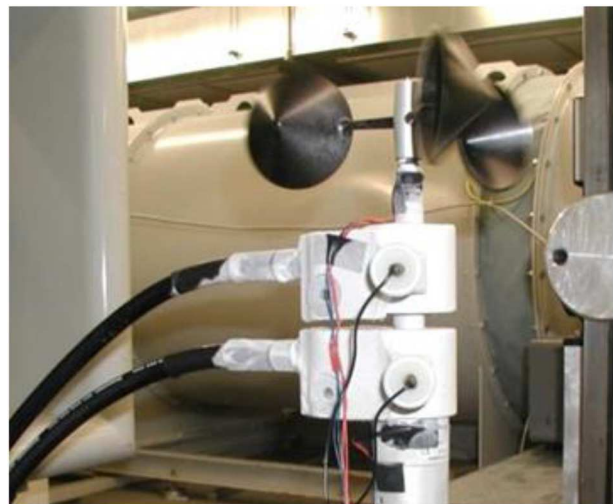
Figure 3: Externally cooled anemometer in the test section. Experimental set-up for producing cold temperatures through the cooling device. The wind is from right to left, and the cup anemometer's housing is surrounded by two cooling devices. For viewing clarity, the necessary thermal insulation is not shown [10].
