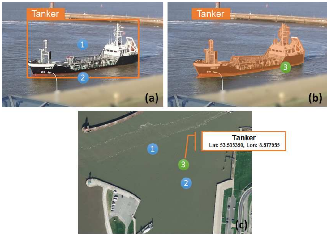
Figure 1.1: Conceptual representation of ship detection, segmentation and georeferencing from maritime footage. (a) Tanker being detected. Point 1 represents the bounding box center, and 2, the bottom-center point. (b) Tanker being segmented. Point 3 represents the intersection of the navigation antenna with the water. (c) Representation of the georeferenced tanker displayed on a map. The georeference from the mask, 3, provides the most accurate ship location of the three points.
