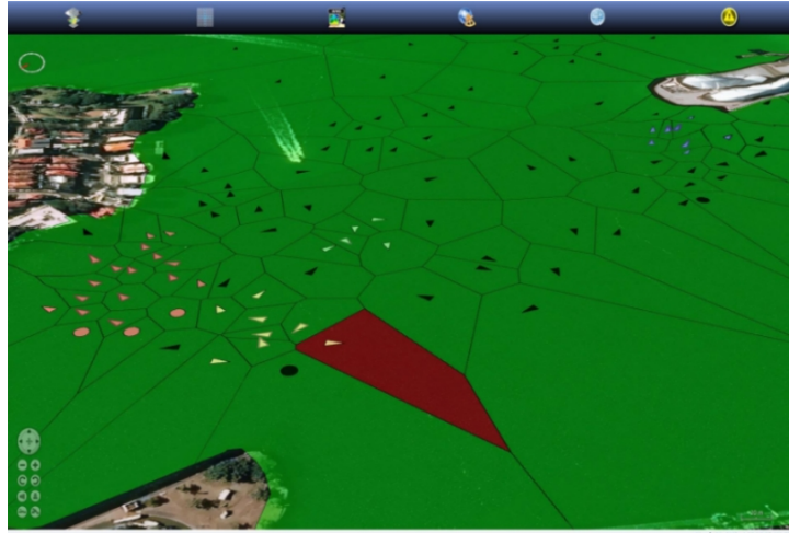
Figure 7.4: Visualization of detected and georeferenced vessels with heading. The vessels detected are provided to a web service map (WorldWind [124]) in the form of triangles pointing towards their motion direction. Vessels for which the motion displacement was near zero are represented by circles. The rest of the figure represents the anomaly detection and visualization pipeline presented in [BCP-I]. The red cell represents the interpreted area in which the anomalous ship is navigating. Reprinted from [BCP-I]. ©2021 IEEE.
