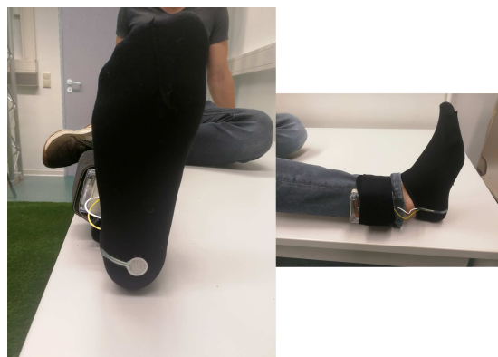
Figure B.2: Attachment of the sensor at the heel and MCU at the ankle.
