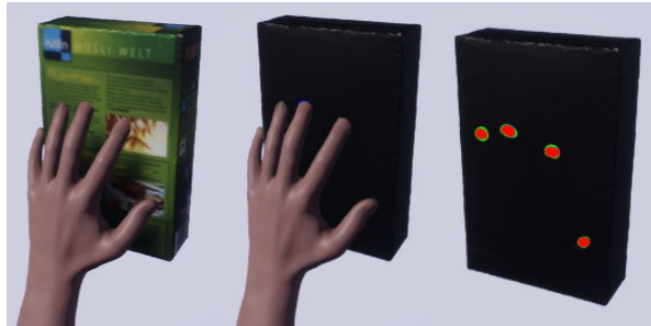
Figure 7.2: The hand grasping the object on the left, the texture for the forcemap in the middle and the final forcemap on the right.
