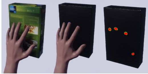
Figure 3: The hand grasping the object on the left, the texture for the forcemap in the middle and the final forcemap on the right.
