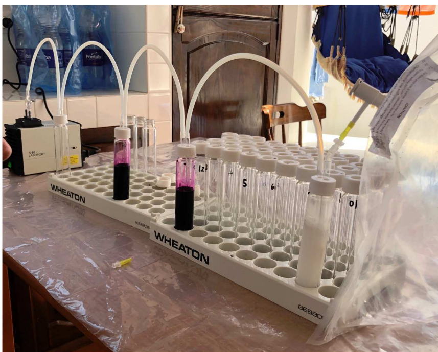
Fig. 5. Impinger train setup with Tedlar® bag to the right, followed by the alkaline and two \text{KMnO}_4 -traps and a vacuum pump at the end (For interpretation of the references to color in this figure, the reader is referred to the web version of this article.).
