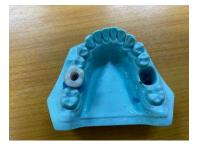
Figure 9.9: Plastic tooth assessment. A plastic tooth #36 is inserted into a dummy dentation. This tooth has correct internal anatomy and convincing physical properties, such that drilling them mimicks the real tooth materials. These teeth can be used once and cost roughly \$10. Additionally, a similarly expensive diamond bur is used to drill them, which also experiences wear.
