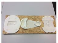
Figure 8.5: Initial dental simulator registration. I first designed the setup to mount the VR controller in the middle. However, it turned out be better to mount it to either side, as it produces more reliable tracking and the distance between the haptic devices can be shortened.
