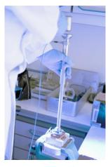
Figure 8.20: Biomedical experimental setup. A donor acetabulum is mounted to a vise, the real implantation tool is hammered into it, while data is recorded.
