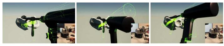
Figure 6.5: Small, complex tool features are also rendered. Sliding the hip reamer across the top surface of the pelvis. The angled reamer head intake (a small bump near the middle along the reamer shaft) collides with the hip and prevents further sliding. Green shows the haptic tool (see Section 6.3).
