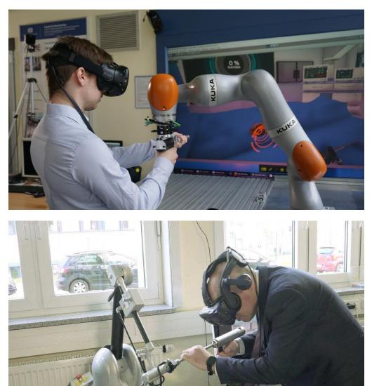
Figure 8.16: HIPS on Haption Virtuose. Showing somone using the HIPS simulator, on a Haption Virtuose.
