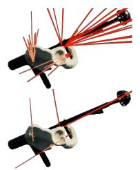
Figure 5.2: Contact clustering. I inserted the acetabular reamer secondary handle into the pelvis cavity and enabled gravity, the tool then settles in this configuration. The amount of contacts (red) is significantly reduced when enabling clustering (*Bottom*). However, the pose is held much more stably when using all contacts without clustering (*Top*), even though many contacts are *seem ingly* redundant.
