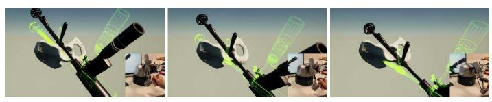
Figure 6.6: Smooth sliding. The other side of the shaft has no such features, and allows for smooth low-friction sliding along the top half of the pelvic bone. Green shows the haptic tool (see Section 6.3).
