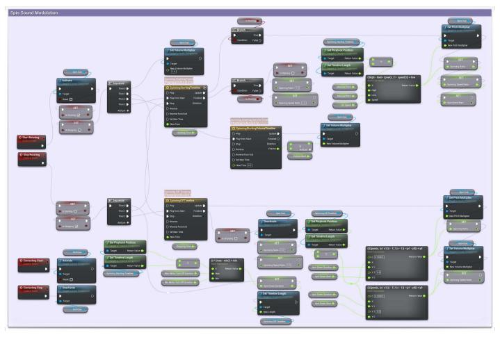
Figure 8.9: Spinning sound synthesis blueprint. The UE blueprint that performs the spinning sample modulation via pitch and volume. When the drill button is pressed and released, the events Start- and Stop Rotation are called, respectively.
