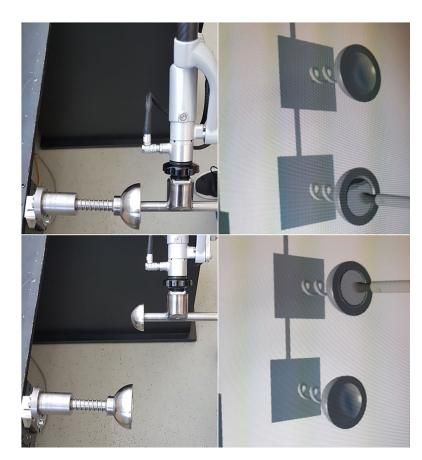
Figure 1. The tool in contact with the real haptic object (top left) and the corresponding virtual view in VR (top right); The tool in contact with the virtual haptic object (bottom left) and the corresponding virtual view in VR (bottom right).
