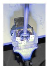
Figure 8.21: Biomedical marker setup. The organ pose is tracked by three markers, and the implant by another marker.
