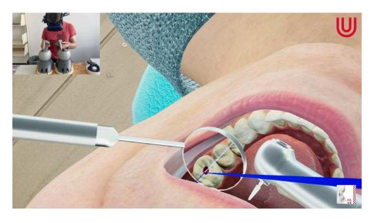
Figure 8.12: Eyetracking in dental simulator. Eye sensors inside the HMD track the pupil position which is used to compute the the gaze direction. The gaze direction is transformed into the UE world and a raycast gives rise to what the user is looking at (displayed as a blue line). Intersections with the mirror are reflected, as that is what the user sees.
