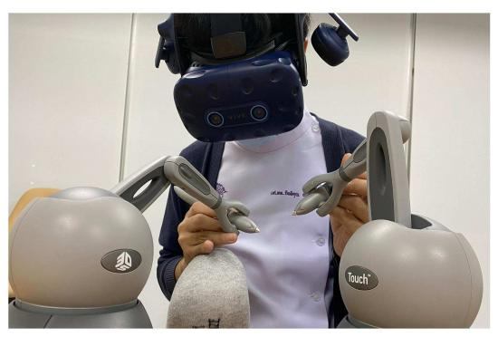
Fig 1. The VR dental surgery simulator is used by a dentistry student to practice root canal access opening on tooth #36. The VR HMD and haptic input/output devices allow for a intuitive control with realistic haptic feedback (in alignment condition). The monitor shows the image that the student is seeing on the HMD.
