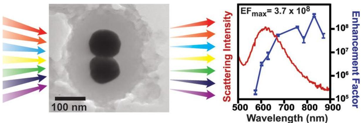
Figure 3.3.2.2 Diagram of scattering intensity (red) and enhancement factor (blue) measured on the single gold nanoparticle dimer encapsulated in a silica shell, with different excitation lasers. Adapted with permission from [219]. Copyright (2013), *American Chemical Society*.
