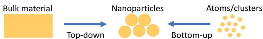
Figure 3.2.1 Schematic representation of top-down and bottom-up approach for the nanoparticle synthesis.
