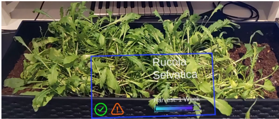
Figure 5.5: Augmentation label for the detected arugula selvatica plants with information on the name of the plant, the duration until harvest, and icons to draw attention to status messages. The label is visualized on the ARCHIE 2 augmented reality interface. [177]
