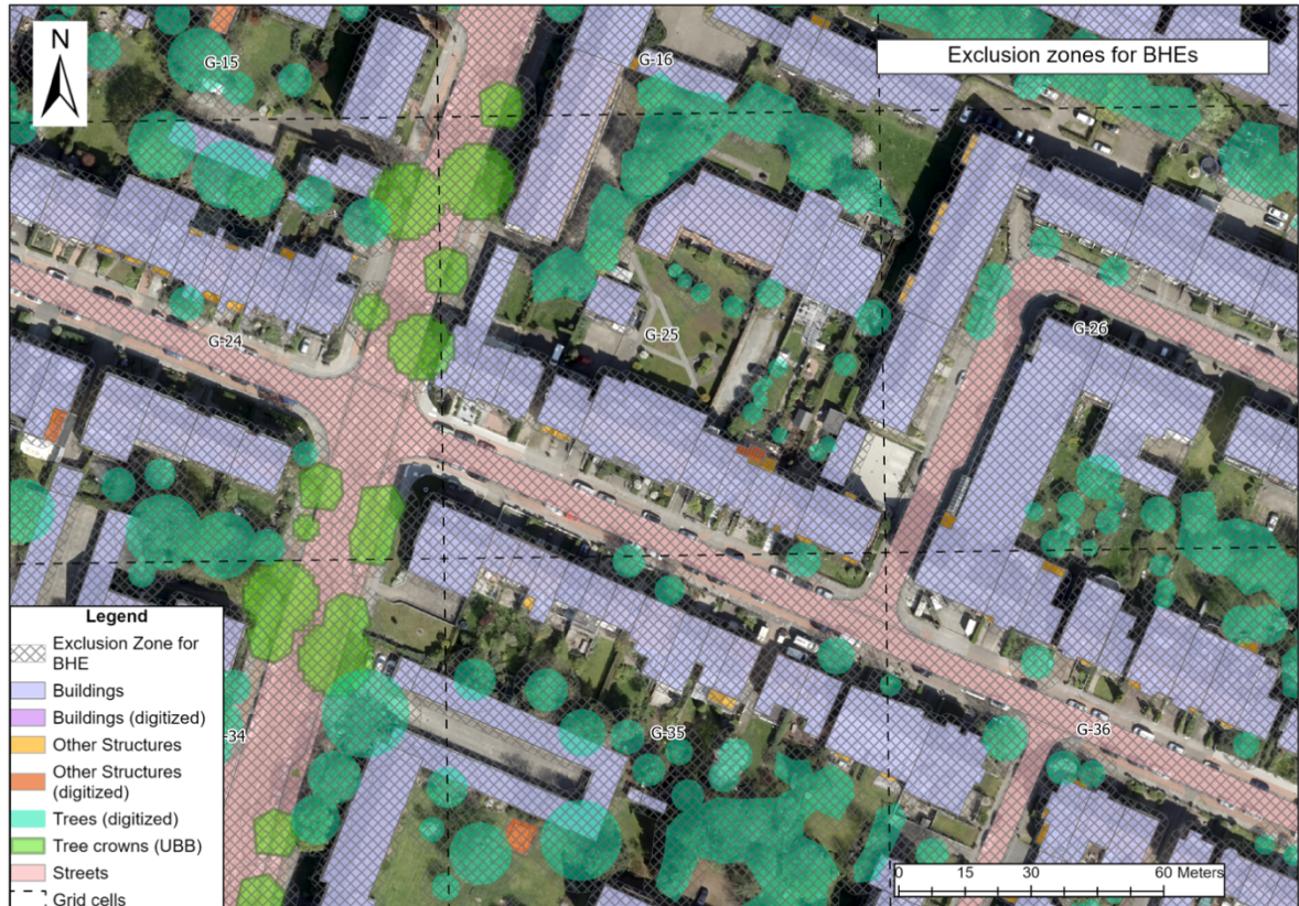
Figure 15: Close-up view of several of the defined exclusion zones for BHEs (Map: DOP10, © GeoBasis-DE / Landesamt Geoinformation Bremen 2023)
