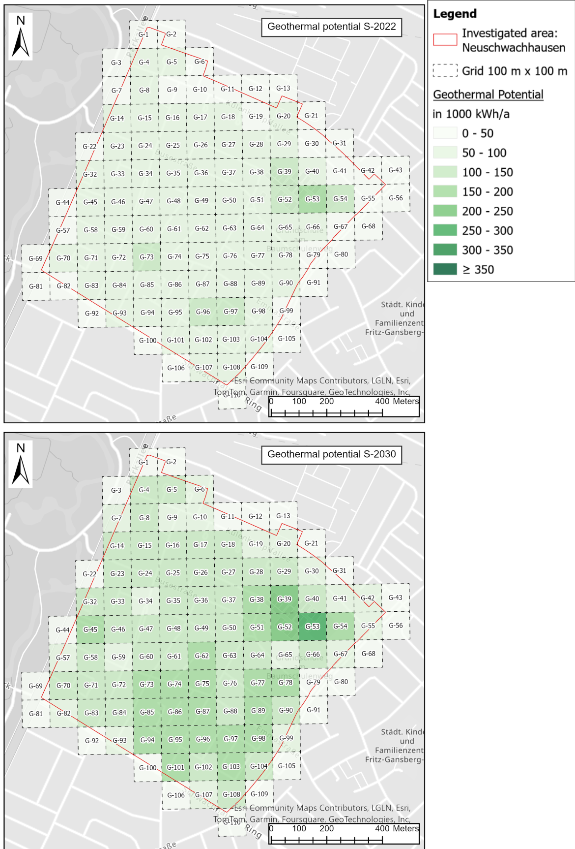
Figure 17: Technical potential of shallow geothermal energy in the scenarios S-2022 (top) and S-2030 (bottom) clustered in grid cells
