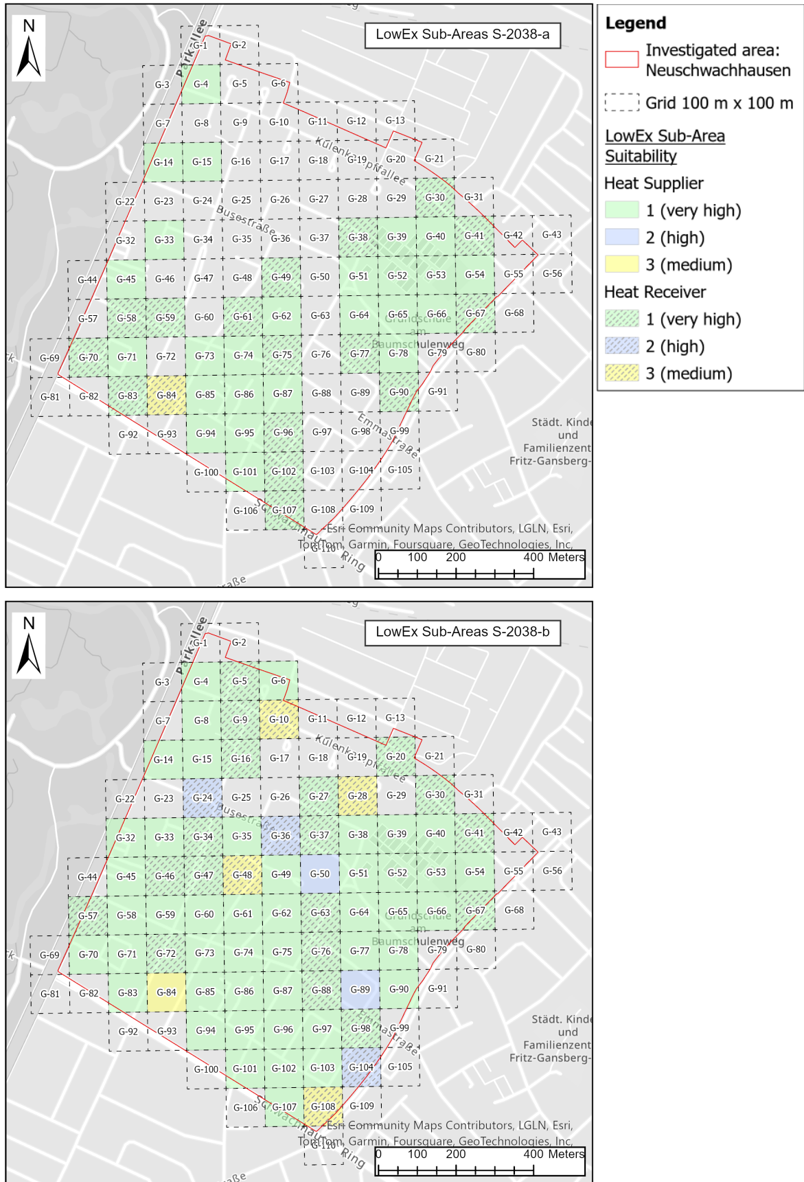
Figure 29: LowEx sub-areas in S-2038-a (top) and S-2038-b (bottom) ranked by their suitability
