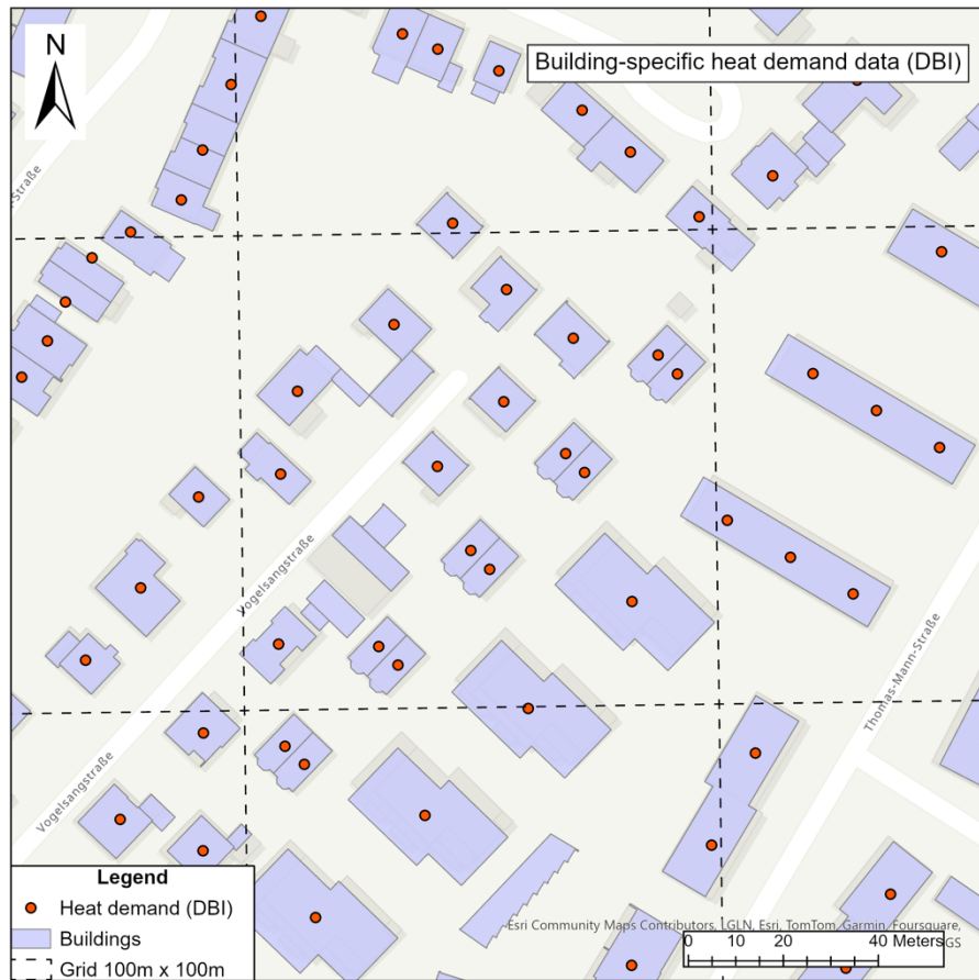
Figure 6: Close-up view of heat demand data (DBI) stored in building-specific points as an example.
