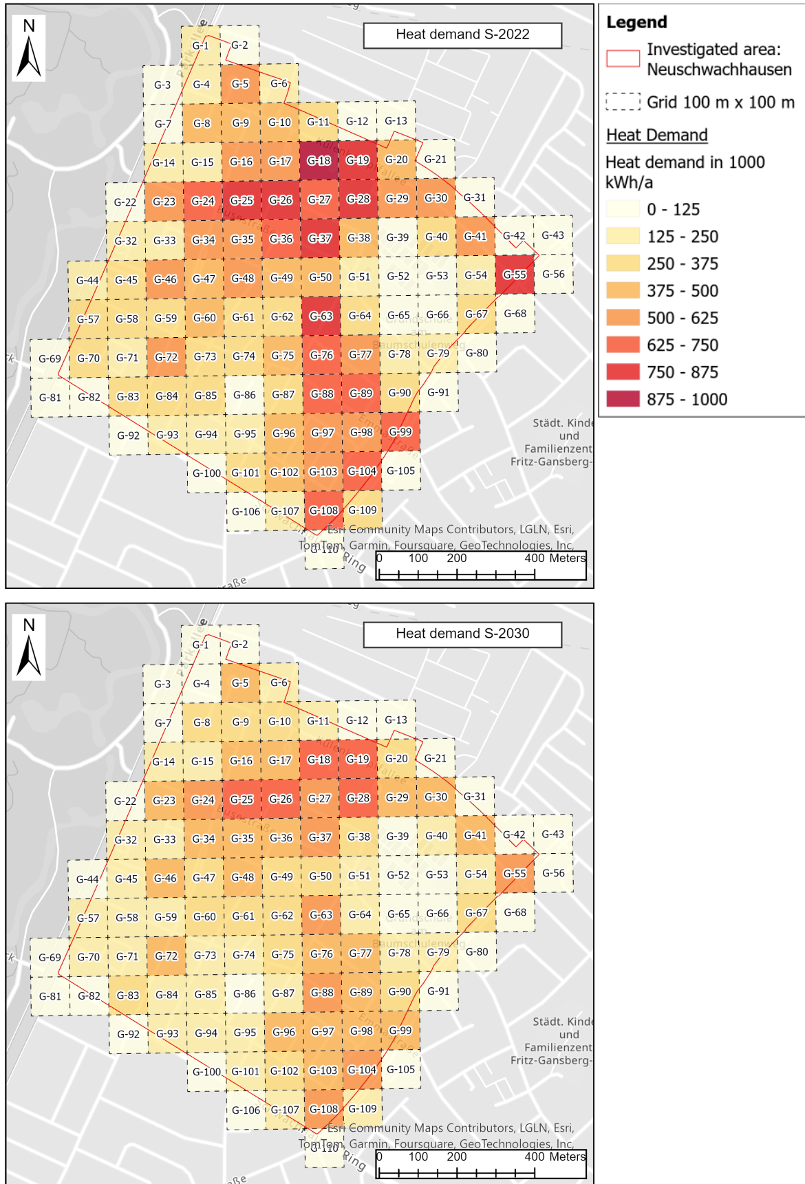
Figure 24: Heat demand distribution in S-2022 (top) and S-2030 (bottom) clustered in grid cells
