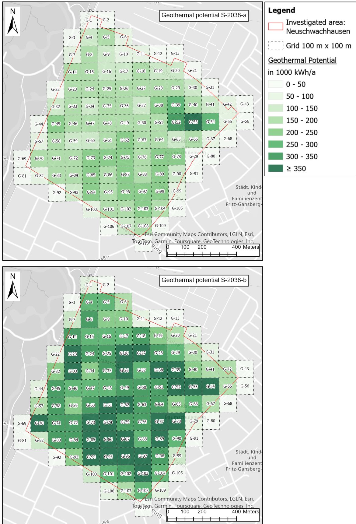
Figure 18: Technical potential of shallow geothermal energy in the scenarios S-2038-a (top) and S-2038-b (bottom) clustered in grid cells
