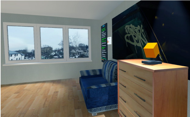
Figure 2: The virtual smart home environment. The voice assistant device on the right is embodied as a hovering cube. Its orange color represents the currently active agent Max responsible for “personal tasks”.
