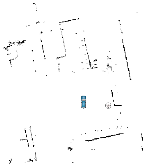
Figure 5.1: Example of an occupancy grid map. The occupancy of each cell is shown in grayscale, with the current pose of the ego vehicle indicated by the blue vehicle.
