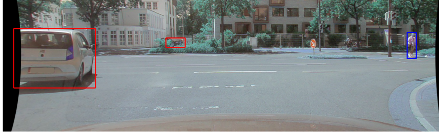
Figure 6.5: Example output of the camera-based object detection overlaid onto the image. Red boxes represent cars while blue boxes show pedestrians.
