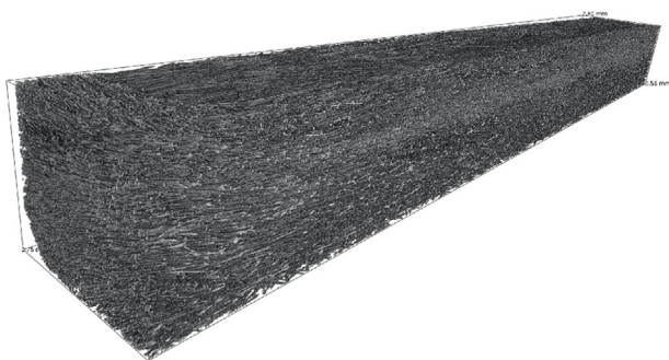
Fig. 7. A3.3, cropped to the plate region, resulting in a 1\,200 \times 8\,832 \times 1\,000 voxel sub-volume. The area closest to the reader is close to an edge where fibers are forced to bend.
