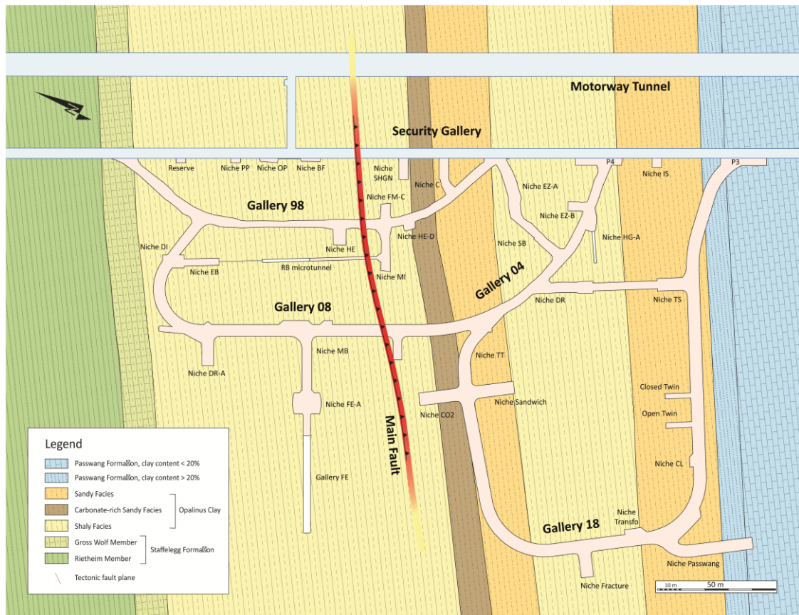
Figure 1.3: Overview of the Mont Terri Underground Rock Laboratory (URL) with indications of different facies within the Opalinus Clay and in situ experiments. The names of the galleries refer to the different stages of construction (1996–2018) and finalization in the URL. The figure was kindly provided by Dr. David Jaeggi (Project Manager of the Mont Terri Project).
