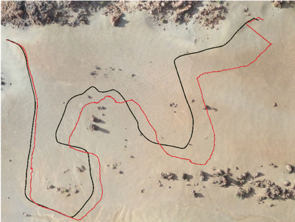
FIGURE 2.4: Estimated positions of a rover traverse using SLAM localization (red) vs ground-truth (black). The SLAM algorithm is able to perform a global pose correction at the end, minimizing the localization error (Geromichalos et al., 2020).
