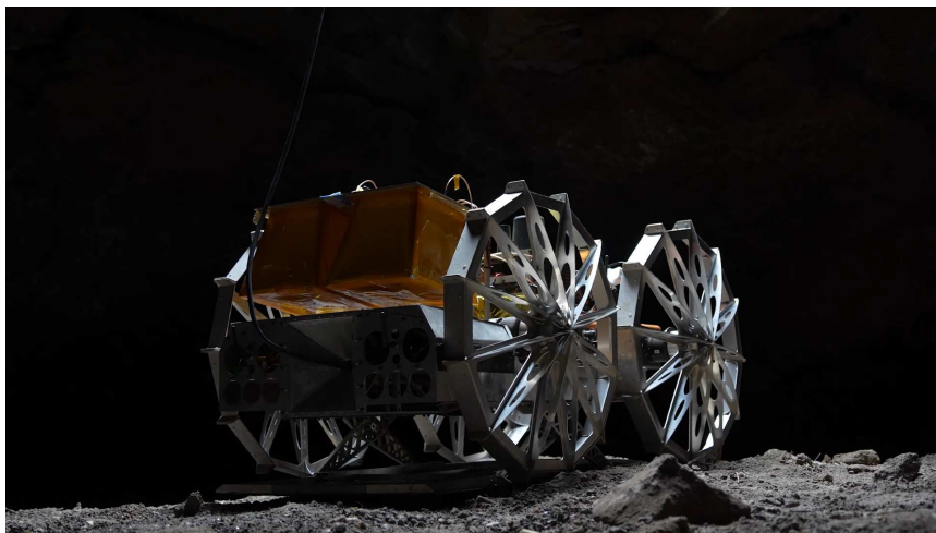
(b) CoyoteIII undocking from the TMDS after successfully landing inside the lava tube (DFKI RIC).
