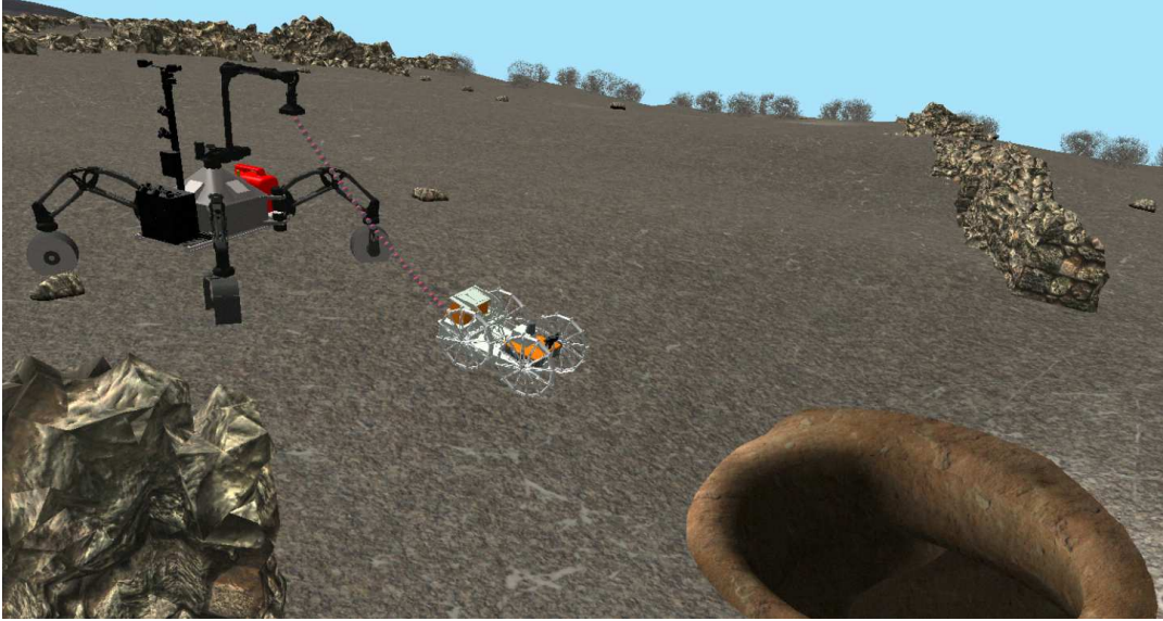
FIGURE 6.25: Snapshot of a MARS simulated rappelling into a lava tube (bottom right), with SherpaTT (left) attached to CoyoteIII (center) by a simulated tether.
