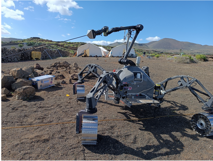
FIGURE 6.29: Final configuration of SherpaTT's robotic arm at the end of a rappelling operation. After the forces are compensated, the arm's last link is perfectly aligned with the tether, thus, the efforts are transferred to the shoulder (joints 1-2) and elbow (joint 3), which are stronger, relieving the spherical wrist (joints 4-5-6).
