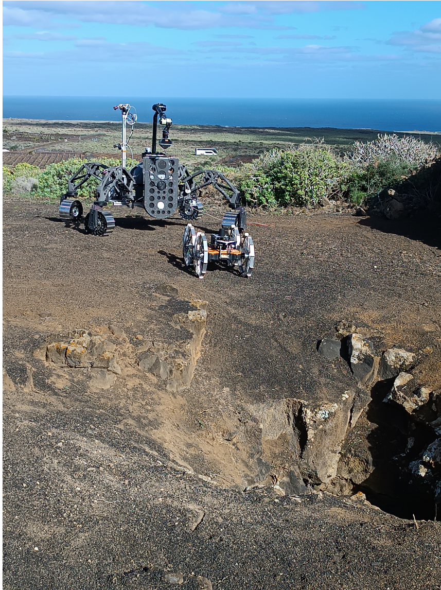
FIGURE 1.7: SherpaTT and CoyoteIII before an attempt to rappel down the lava tube skylight within the field trials of the H2020 CoRob-X project in Lanzarote, Canary Islands, Spain.
