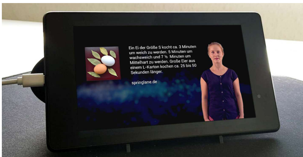
Figure 1: Our prototype of a smart display with an embodied voice assistant agent performed by an actress
