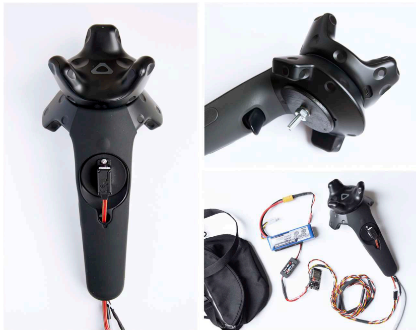
FIGURE 7 | (left) Our haptic VR controller Triggermuscle. (top right) Attachment of the HTC Vive tracker to enable spatial tracking. (right bottom) Electronic components (MCU, the battery and the BEC) are carried in a small bag.
