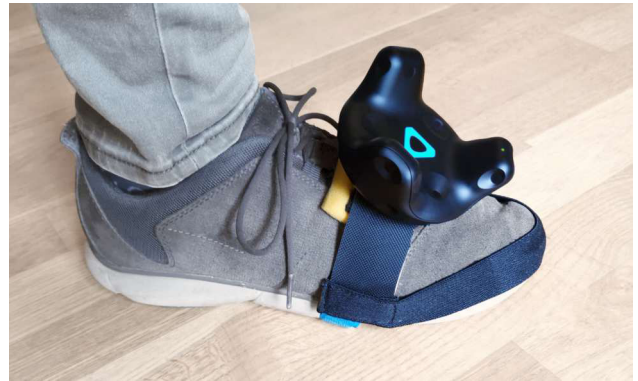
Figure 2: As shown in this illustration an HTC Vive Tracker 2.0 was attached to the top of the players’ right shoe with elastic bands.
