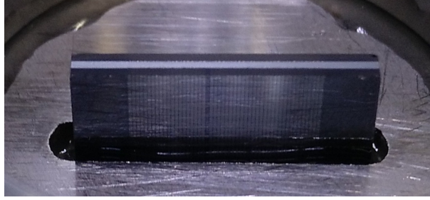
Figure 4.1: A stack of channels glued into a metal socket. A single channel is filled with water, visible as a darker vertical line near the center of the stack.
