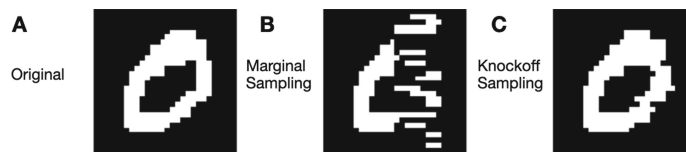
Fig. 1. Sampling of out-of-coalition features for a digit from \{28 \times 28\} mnist data. The first 14 columns from the left are in-coalition, whereas the remaining 14 columns are sampled either from marginals (as in Kernel SHAP [17]) or deep knockoffs [21].
