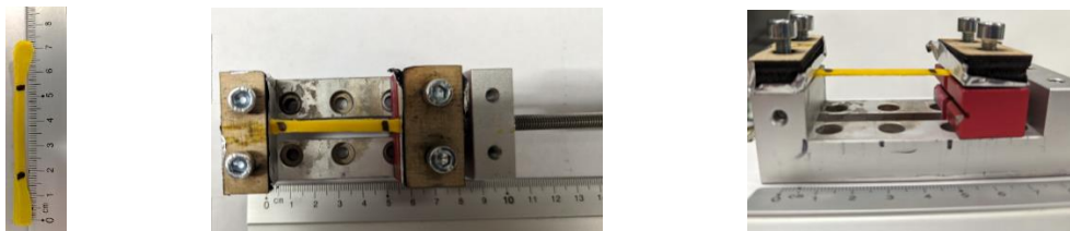
Figure S7: Images of stretched LCE after taken out of the oven.
