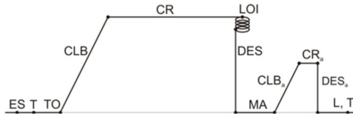
Figure 8 - Typical flight mission phases (Scholz, 2002).
