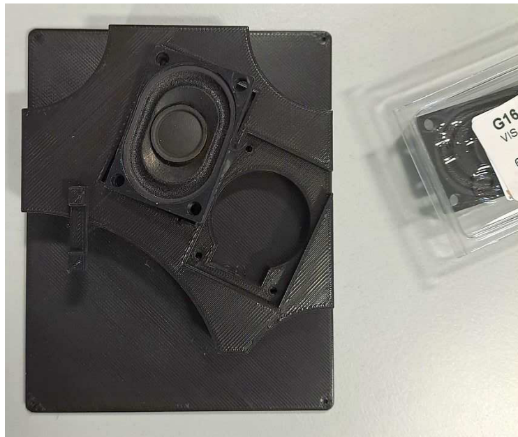
Figure 4.1: 3D-printed mount for the speakers. (photo: Winfried Sembritzki)
