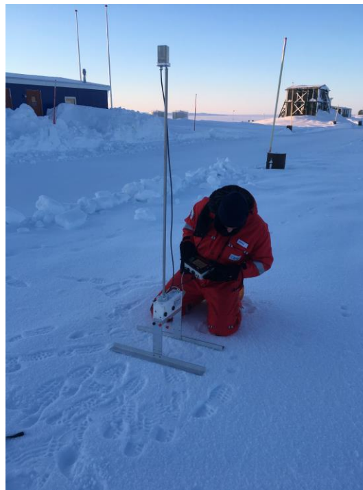
Figure 4.5: Preparation of the SnowMicroPen at Villum Research Station, Greenland (Photo: Andreas Herber).
