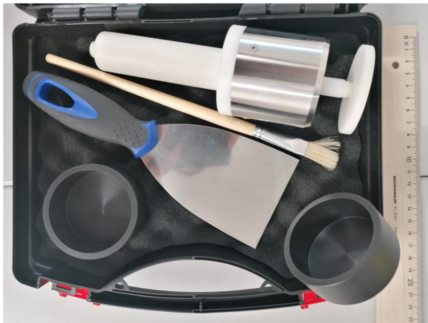
Figure 4.4: Snow sample holder for IceCube measurements and tools to receive the snow sample (Photo: Daniela Krampe).
