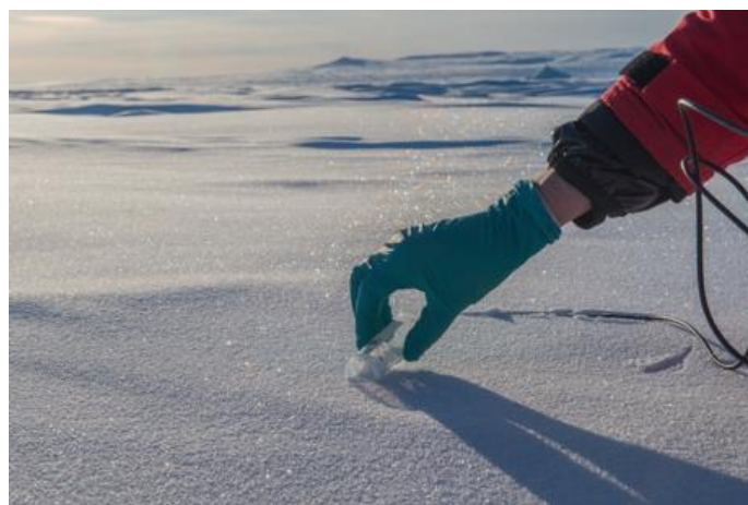
Figure 9.2: Sampling of surface snow for later analysis of black carbon (BC) concentration during PAMARCMiP (Polar Airborne Measurements and Arctic Regional Climate Model Simulation Project) 2018 (Photo: Andreas Herber).
