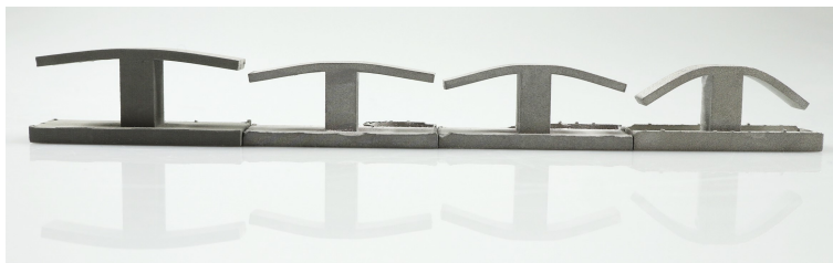
Figure 6.30 Example of the deflected T-shape samples with IRD of 58% at sintering temperatures of 1050 °C, 1150 °C, 1250 °C, and 1350 °C (from left to right).
