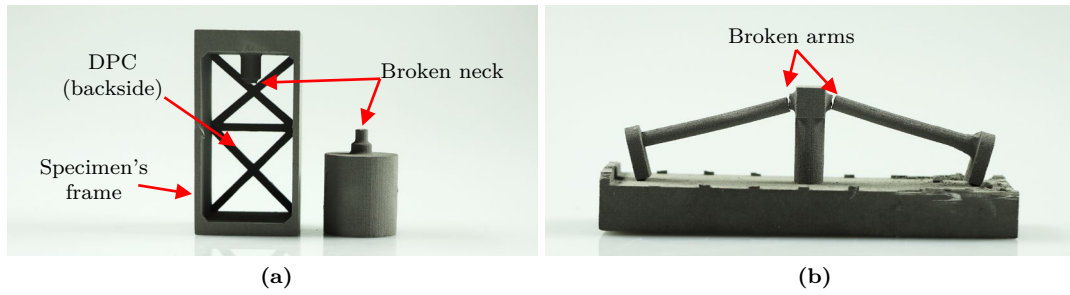
Figure 5.6 Two broken specimens (a): a tensile specimen and (b): a bending specimen.
