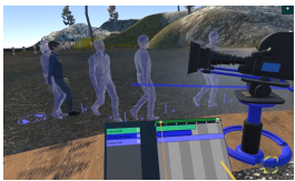
Figure 2: Character walking animation can be performed by grabbing a node with the handheld controller and drag it across the scene.
