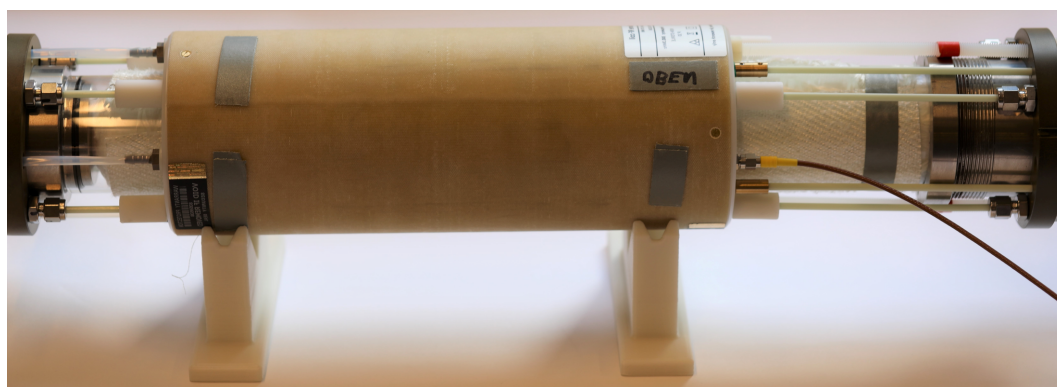
Figure 3.1: Image of the original reactor built for MRI applications and the specially designed RF coil by MRI.TOOLS. Reprinted from [1] under creative common license (CC-BY 4.0).
