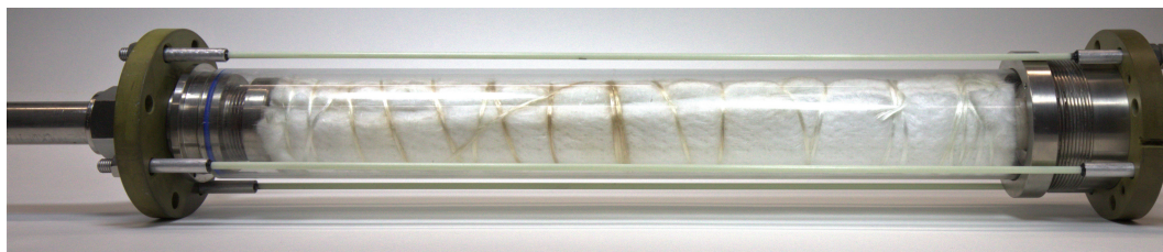
Figure 3.2: Image of the MRI reactor with the new inlet featuring a larger tube. It is designed for frontal heating of the reaction using an unfocused laser. A detailed view of the changes between the two reactor designs can be found in Figure B.1.
