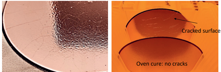
Figure II.20: Photoresist cracks during hotplate prebake. No cracking occurs with oven curing. The right figure indicates a wafer with oven curing (front, without cracks), and hotplate curing (back).
