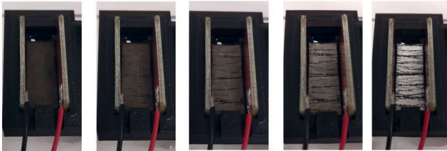
Figure IV.16: Carbon nanotube alignment in DI-water as Proof of Concept. The electrodes (1cm apart) are placed directly into the solution.
