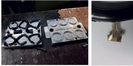
Figure V.3: Preparing the sealings and for integration. (a) HNBR pieces are placed inside the mold, just before the first vulcanisation step. (b) Final integrated sensor inside the sealing.
