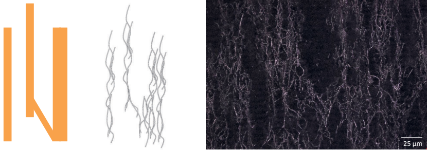
Figure VI.4: No real idealised uni-directional alignment is possible. There are always some cross-overs when utilising pristine multi-walled carbon nanotubes.
