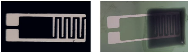
Figure III.5: Screen-printed inter-digital electrodes (left). CNT-PDMS composite mold-printed on top of electrodes (right). For clarification purposes a 0.2 CNT wt% solution was printed in order to leave the electrodes visible through the layer.
