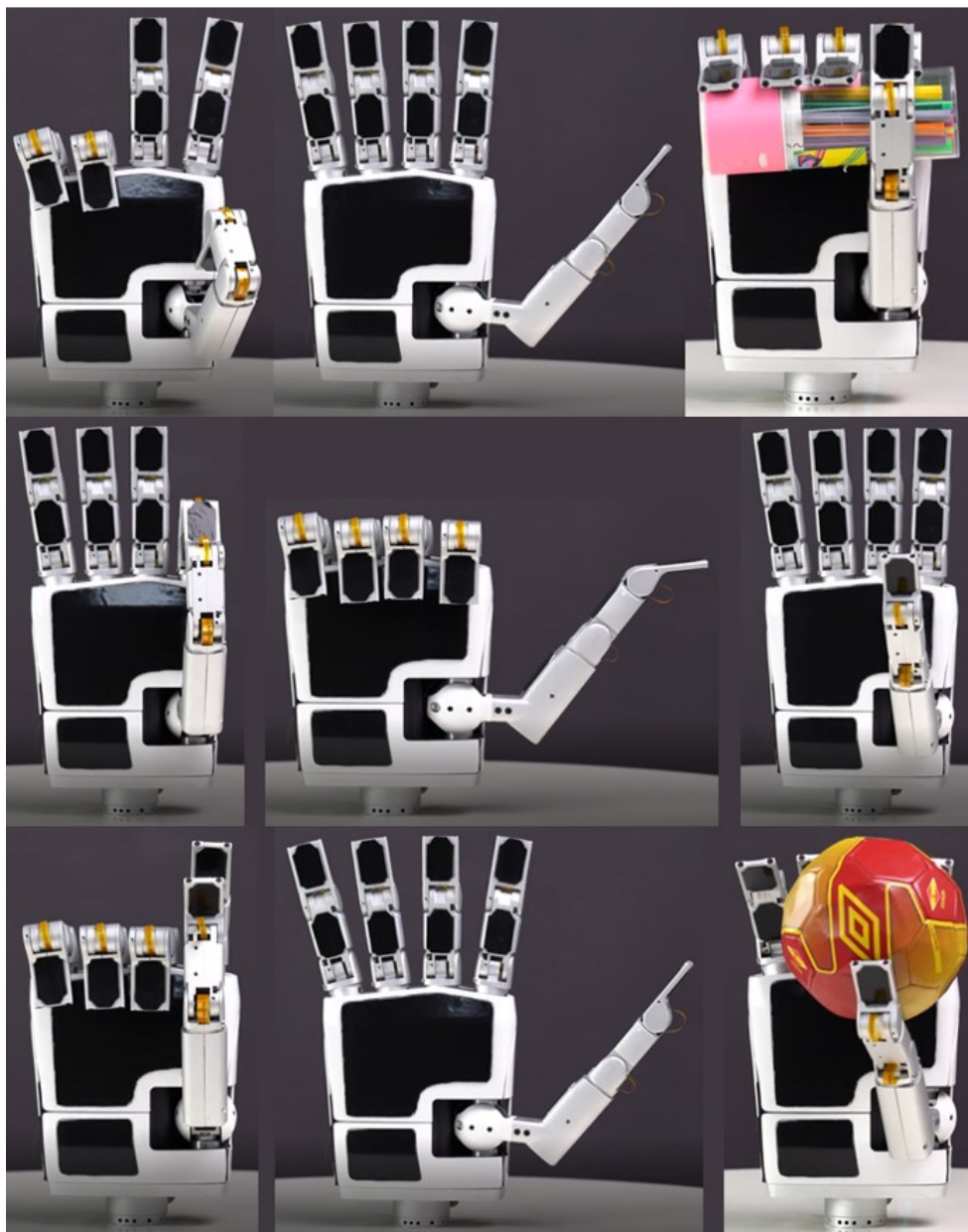
Figure 4.11: Different gestures and grasp poses with five-finger hand
