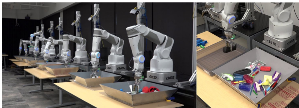
Figure 2.16: Collecting grasping data with fourteen robots
