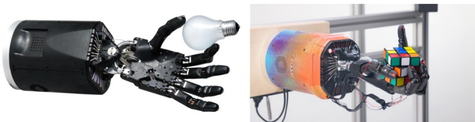
Figure 2.1: Shadow Dexterous Hand and application with Rubik's cube
