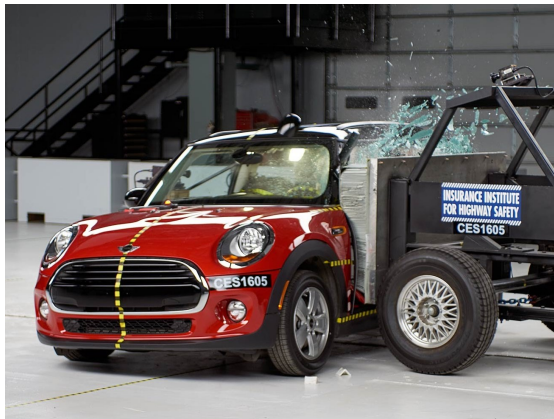
Figure 3.2: 2016 MINI Cooper side crash test using an aluminum honeycomb analog for an impacting car (courtesy of: www.iihs.org )
