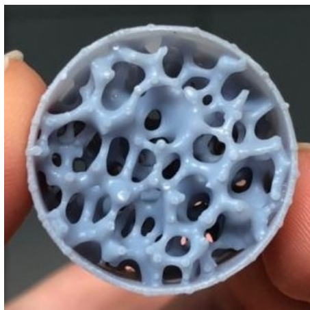
Figure 13: From the stl-file shown in fig. 10, an OCF structure was 3D-printed of PLA and used for the measurements. For details, see table 1.
