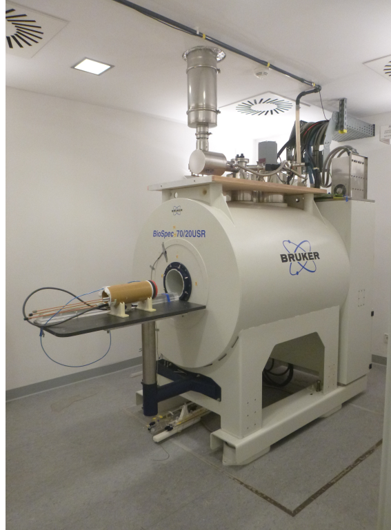
Figure 7: The MRI scanner BioSpec 70/20 USR and the unmounted birdcage coil.
