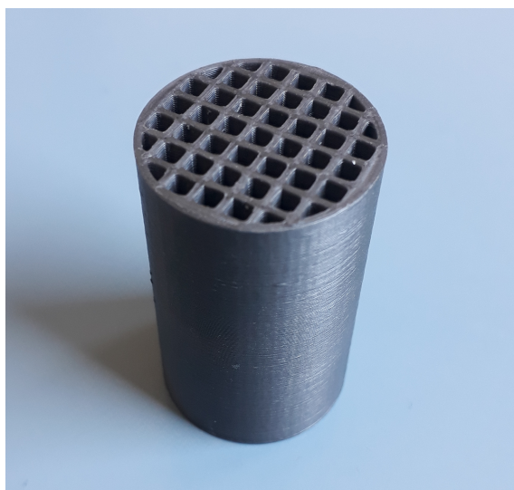
Figure 16: A honeycomb structure made of PLA used for the measurements.
