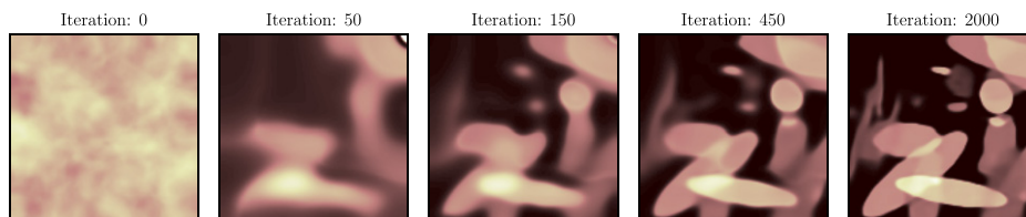
Figure 3. Intermediate reconstructions of the DIP approach for CT (ellipses dataset, see section 6.2). At the beginning the coefficients are randomly initialized from a prior distribution. The method starts reconstructing the image from global to local details.
