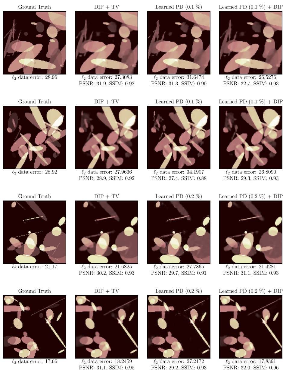
Figure 12. Examples of reconstructions obtained with the DIP approach combined with TV, the learned primal-dual method trained with 0.1% and 0.2% of the Ellipses dataset (32 and 64 resp. data-pairs) and the DIP approach with initial reconstruction. The \ell_2 data error measures the discrepancy between the noisy observation and the noise-free projection of the (reconstructed) image.
