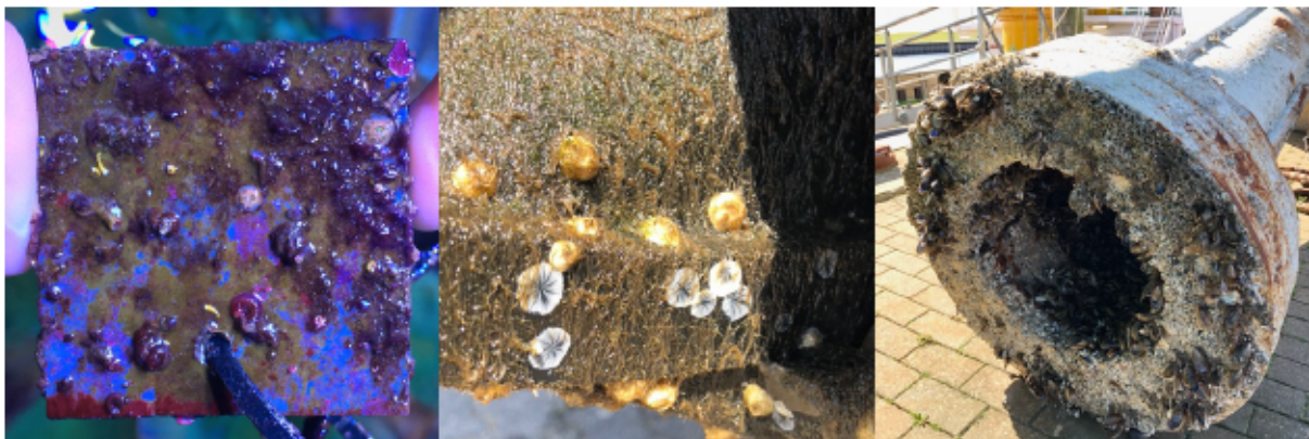
Figure 1.2: Polyvinyl chloride (PVC) tile overgrown with soft and hard fouling organisms; incl. coral spat after 3 months in a seawater aquarium at ZMT (photo left). Leisure boat's hull overgrown with algae and barnacles after one season in the German Baltic Sea near Kappeln (photo center). Mooring buoy overgrown with barnacles and blue mussels after one season in the German North Sea near Husum (photo right).
