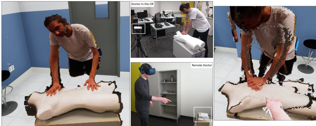
FIGURE 3.2: Example of our system. Left: Live-streamed point cloud visualization of the local doctor in the real OR, seen from the perspective of a remote doctor. Middle: Physical environments of the local (top) and remote (bottom) doctors with RGB-D cameras (see white rectangles). Right: Point cloud visualization of the local doctor using two cameras to minimize occlusions, and part of the remote doctor's self-avatar.
