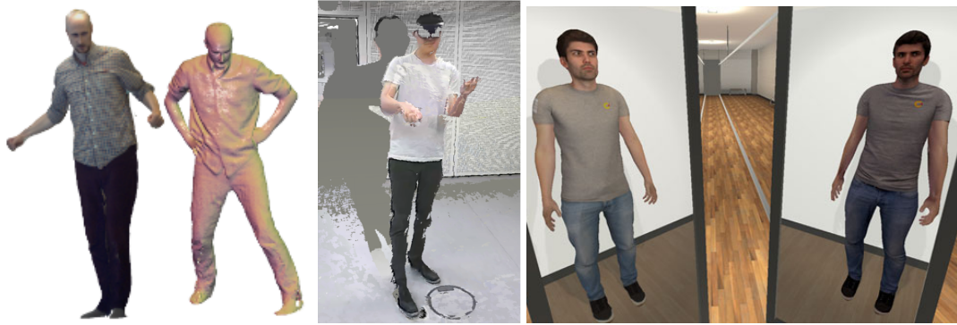
FIGURE 2.9: Various scene/avatar reconstruction methods. Left: real-time volumetric RGB-D-based mesh reconstruction [91]. Middle: real-time point cloud rendering [431]. Right: high-cost and low-cost offline 3D mesh reconstruction [18].
