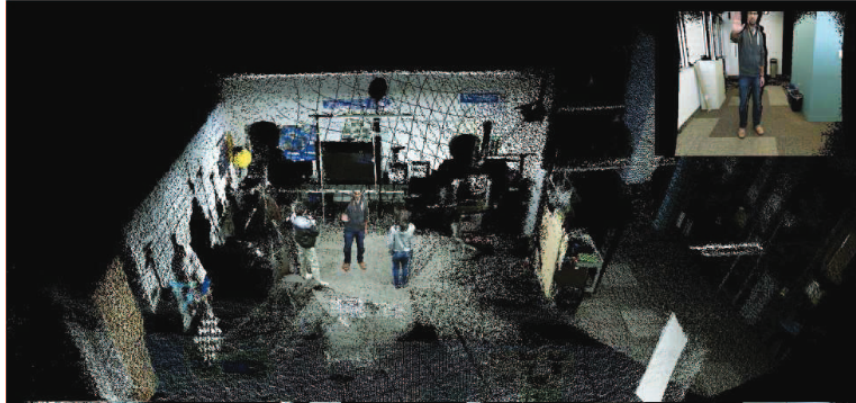
FIGURE 2.10: Example of a small-scale environment, which gets live-captured by multiple RGB-D sensors and rendered using point clouds [361].
