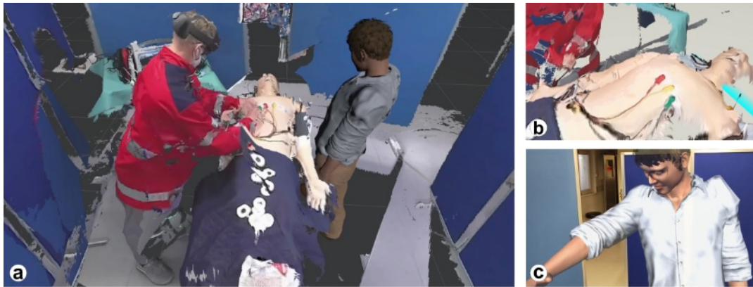
FIGURE 2.13: A MR telepresence application. a: third-person view of the real-time 3D-reconstructed environment including the remote expert's avatar (right). b: first-person view of the remote expert on the virtual patient. c: remote expert's avatar as seen by the local participant. [359].
