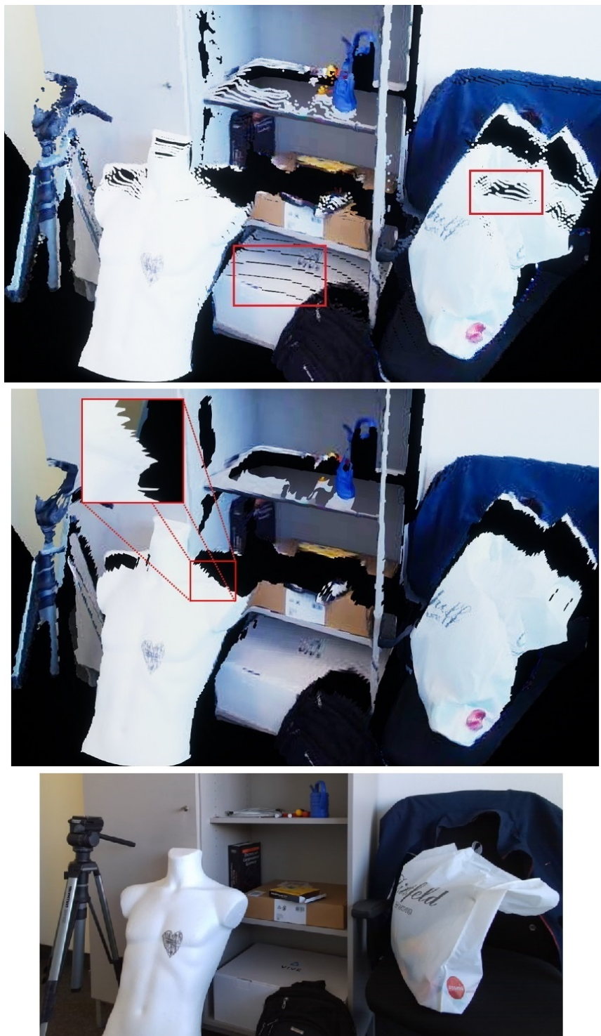
FIGURE 3.6: Comparison of the two point cloud renderers, splatting in the top, fast mesh reconstruction in the middle. Both look quite good but the splatting method still has visible holes in some areas, see the red rectangles. With the mesh, however, object borders can look jagged (see highlighted region). The bottom image shows the captured scene.
