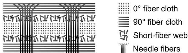
Fig. 1. Schematic representation of the 2.5D fiber reinforcement in the prepared 2.5D C/C-SiC composite.
