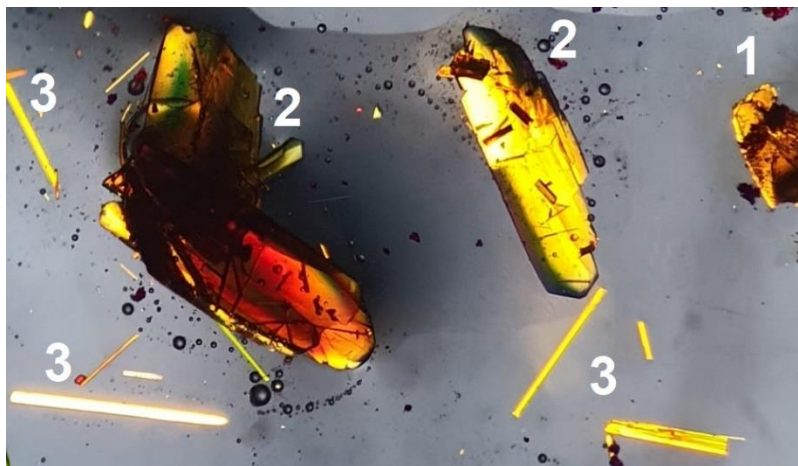
Figure 108: The three obtained crystal types after 2 nd crystallization cycle: 1) literature known \text{ReCl}_4(\text{PPh}_3)_2 ; 2) starting material \text{ReCl}_3(\text{CH}_3\text{CN})(\text{PPh}_3)_2 ; 3) (endiolato) \text{ReCl}_2(\text{PPh}_3)_2 ( 118 ).
