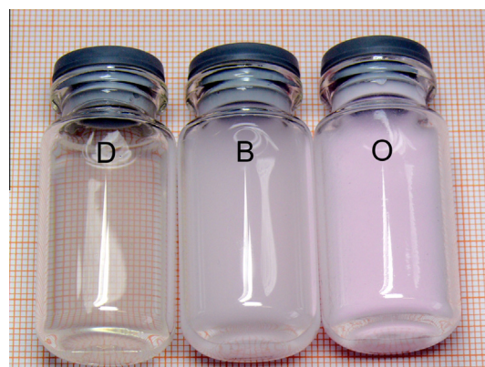
Fig. 4. Typical samples after filtration experiments. O: Original Sample, B: Backwashing Sample, and D: Sample after DEP filtration.
