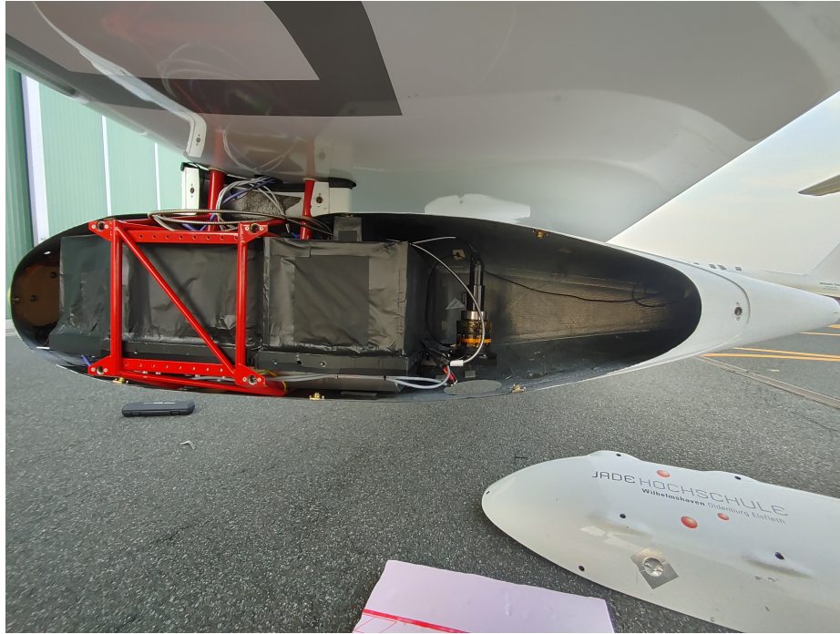
Figure 5.4.: Mounting of the MAMAP2D-Light instrument inside the wing pod of the Dimona motor glider. The spectrometer is covered inside a matt black, light tight aluminum foil housing, the electronics are mainly mounted below the base plate.
