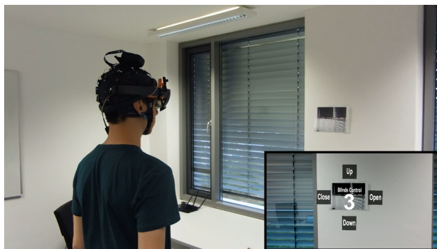
Fig. 1. Window blinds control via AR using the SSVEP-BCI paradigm in a room where the menu allows for four operations: blinds up, blinds down, blinds close (fins), blinds open (fins) – the operations are automatically executed via the building’s intelligent control system.
