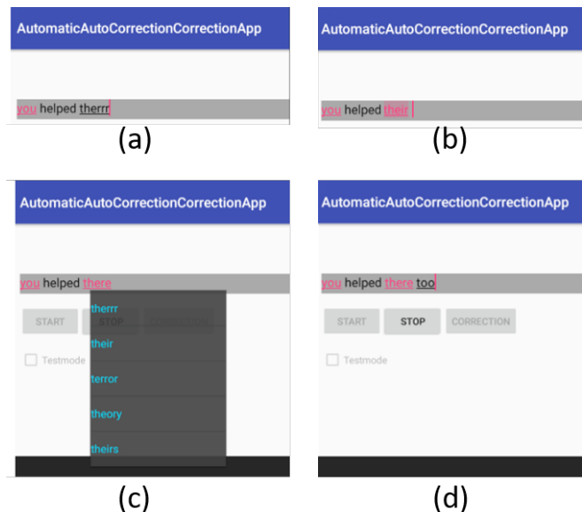
Figure 6. Screenshot of the user interface for the text entry with automatic self-repair, showing the user making a text entry error (a), an auto-correction error (b), an automatic self-repair with a pop-up (c) and the result after a finished self-repair (d). Example in English for illustration purposes.
