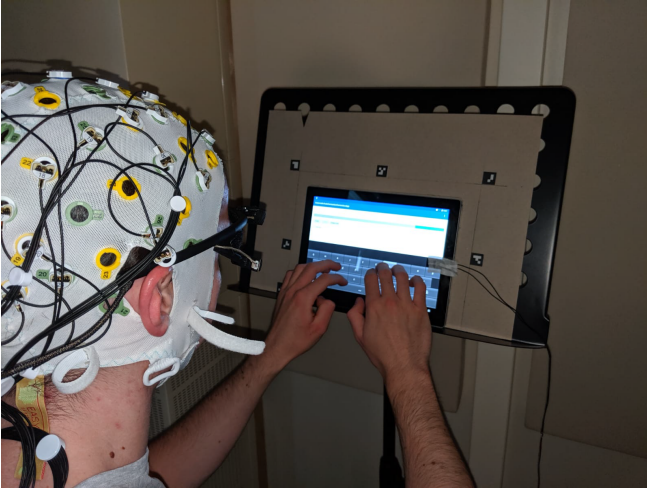
Figure 7. User typing on Android phone using self-repairing auto-correct in the experimental setup with EEG cap and eye tracker.
