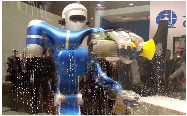
Fig. 1 The humanoid robot Rollin' Justin wiping a window as a demonstration for a compliant whole-body task.
